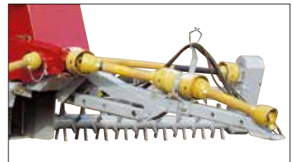
The depth is controlled by an articulating drawbar.
