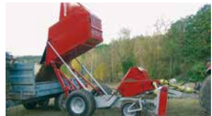
The hopper has a tipping height of 2.3 metre.
