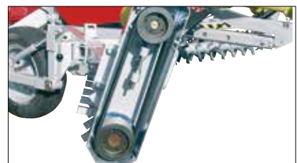
A V-belt pulley powers the stone rakes.
