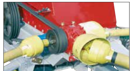
The rotor is powered by a reversing gearbox and a straight V-belt pulley.
